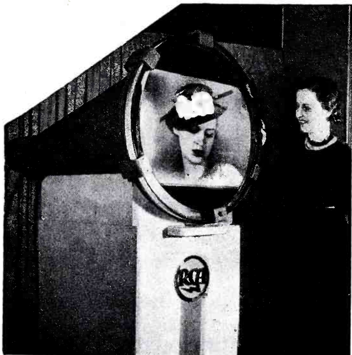
▲ Above—Special large size cathode ray tube built in the RCA television laboratory at Camden, N. J. Aside from the fact that an extra large image is produced on the fluorescent screen, this tube differs from the ordinary one in that it has an automatic pump to maintain a high degree of vacuum within the tube.
