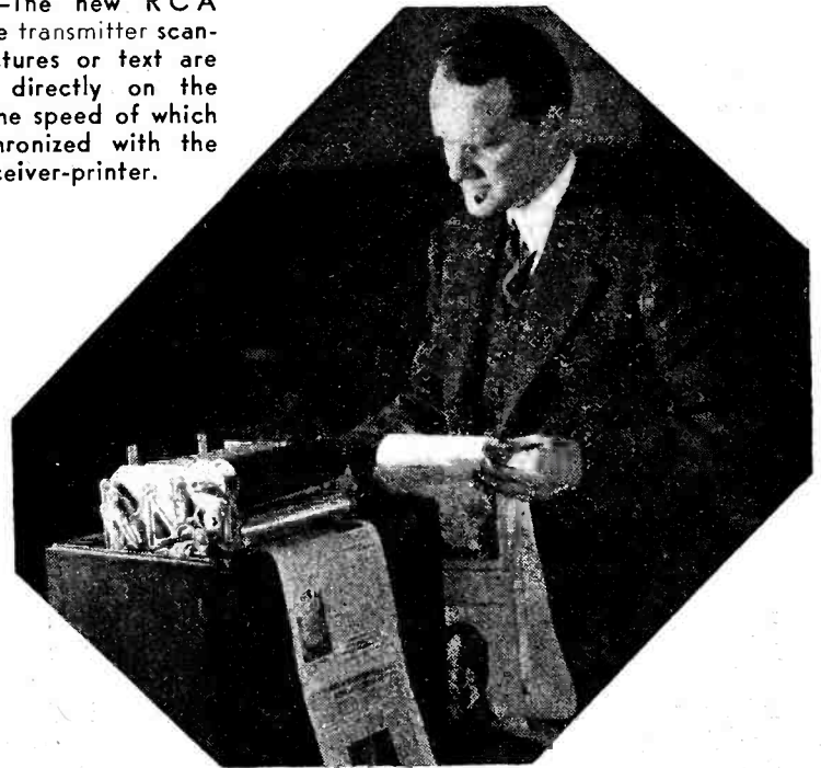
Above—Charles J. Young, RCA engineer, with the simplified facsimile receiver-printer with the lid-cover removed. Ordinary white or newsprint paper and carbon paper are utilized for reproduction.
