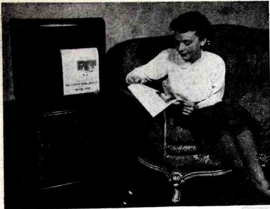
The RCA facsimile receiver. All the controls are within the cabinet, so that they may not get out of adjustment. 8½- by 12-inch pages on a continuous roll are printed at the rate of three feet an hour.
